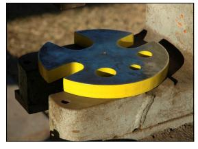
completely. Someone's "Plan B" was to add support by the use of an under plate. That's not a bad idea but the support was only  $\frac{3}{4}$ -inch plate and it seemed marginal to me. I secured a hunk of 1  $\frac{1}{2}$ -inch plate and went to work matching size and existing bolt locations. This is the kind of \$5 project that is accomplished by using \$5,000 worth of tools.
