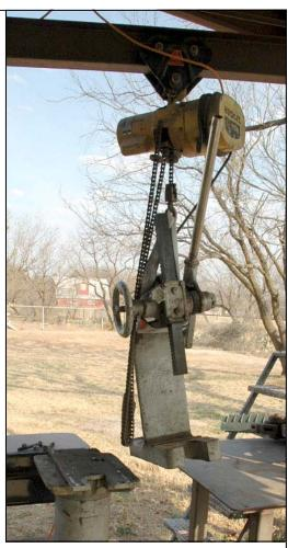
Next, The press is lifted off with an electric hoist, the old support discarded, and a trial fit made on the new support. Then, the mounting holes are drilled in appropriate locations by spotting through existing
