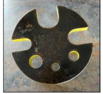
As a final step, I disassembled the parts that move, cleaned and lubricated everything, and fabricated a missing gib plate for L-R ram clearance adjustment.
