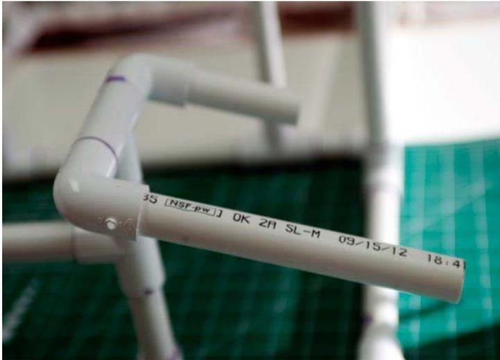
Here's the gear support. I use a droop on the legs. The long piece is use to help align the angles of the droop on the front and back. After aligned the pieces are cut so about a 1-1/2" is left. I then add a cap to finish the ends.
