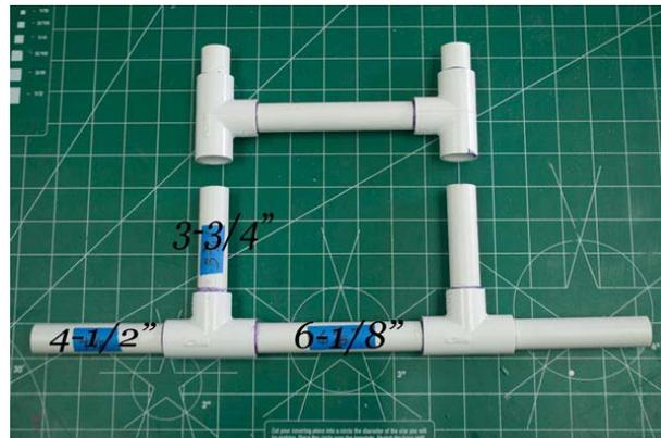
The 90 degree elbows determine the vertical alignment. As you can see in the photo, I use a square to set the angle of the elbow before it is glued. You can then mark an index line on the horizontal piece and the elbow. Now adding the elbow and getting the verticals to actually be vertical is much easier. Simply add glue and align the index mark.
