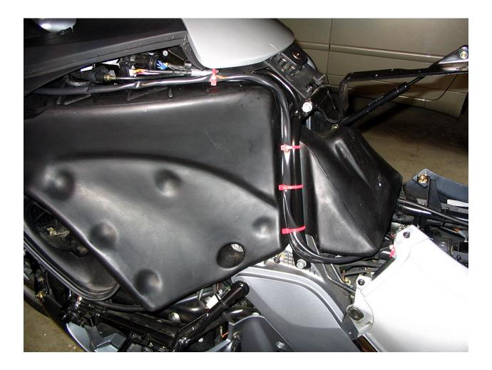
From the gas tank top, route the connector-end of the harness inboard of the steering head and between the fork tubes along the front sub frame center spine, again following the path of the existing wiring harness.
