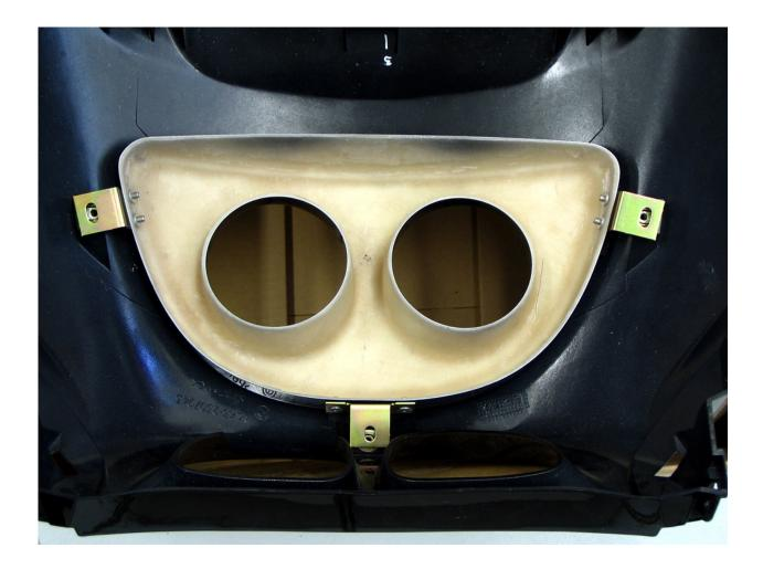
Install the headlight module in the nosecone behind the nacelle. It should fit loosely in the nacelle, with plenty of adjustment range in the mounting tab holes.
