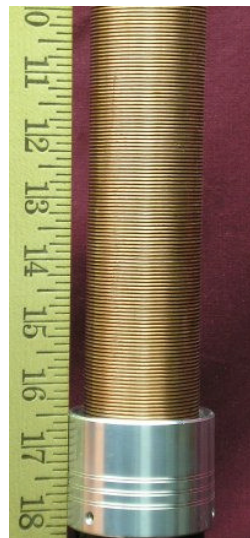
Model 400 -- 8.8 MHz with 5 ft. whip and 16 1/2" of coil showing
