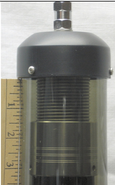
Model 40A-HP -- 14.2 MHz with 5 ft. whip @ 1/2" of coil showing
